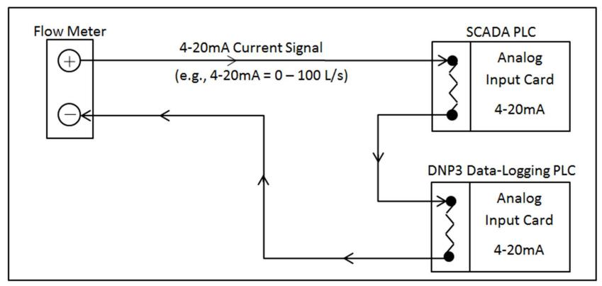
Wiring the DNP3 data-logger using the "wiring-into-the-loop" feature of 4-20mA analog signals.
