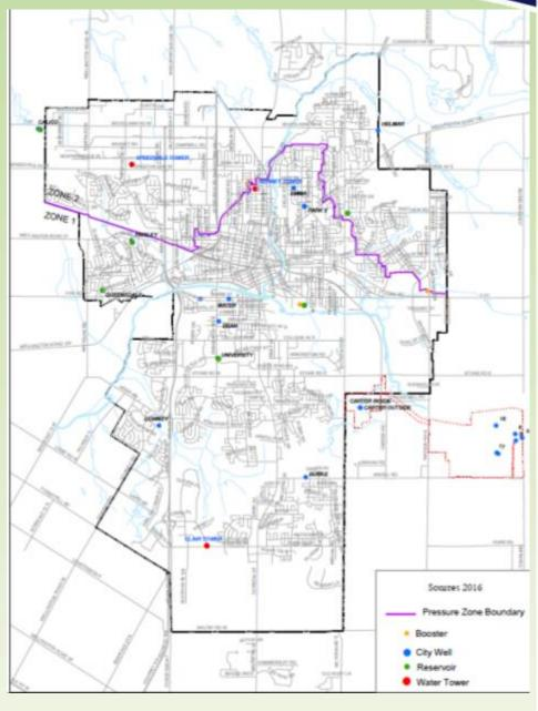
All sites are linked together with SCADA Network for remote control, automatic control, monitoring and logging.
